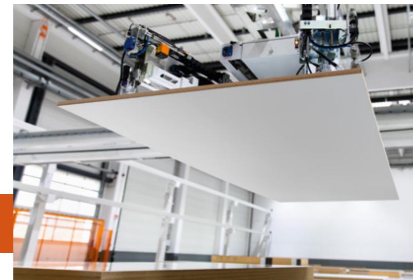
Compressed air is required for the suction machines that are used to lift large production pieces (via the Venturi principle).
