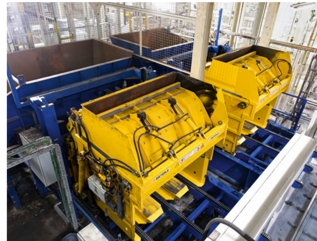
Preparation and charging for the coating of pourable bulk materials takes place in these lifting-and-tilting devices (drum processing).
