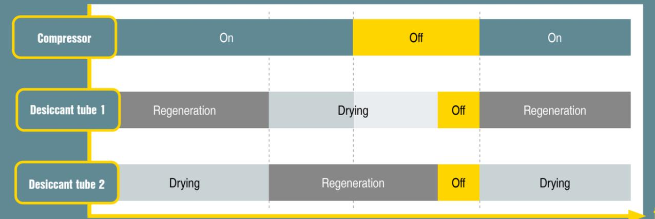
Upon receipt of a 'Remote Off' signal, the currently running regeneration phase is fully completed. Only then does the half-cycle end. This requires dried compressed air. The next half-cycle starts when the 'Remote On' signal returns.
