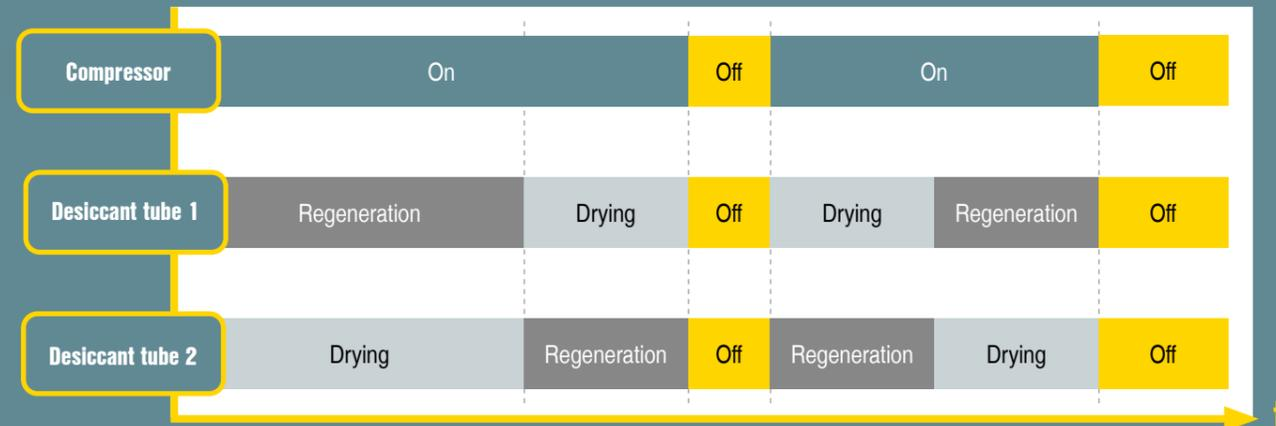
Upon receipt of a 'Remote Off' signal, the cycle will be stopped immediately. Upon receipt of a 'Remote On' signal, the cycle will be restarted.
